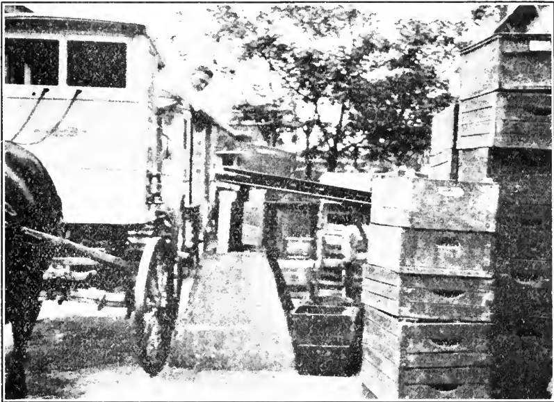
FIGURE 6.—Unloading bottles on a conveyor at a plant using system 2. An average of 22.5 routes per hour and 8.1 routes per man-hour was checked in at eight plants using this system
